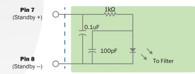
Figure C: An equivalent circuit looking into the STANDBY pin.
