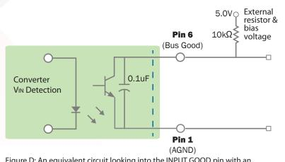
Figure D: An equivalent circuit looking into the INPUT GOOD pin with an example external pull-up circuit.
