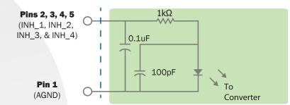
**INHIBIT Controls:** EachconverterhasanindependentINHIBITcontrol,shown
